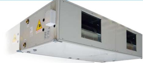
The frame is made from steel profiles and the panels are sandwich type, with thermal and acoustic insulation in mineral wool (10 mm thickness for 10 to 40 model, 20 mm thickness for 50 and 60 models). The panels are prepainted galvanized steel outside, galvanized steel inside, supplied with gripping seals fixed to the frame by steel screws.
